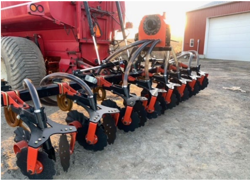
Figure 18. Manure injection toolbar attachment to inject manure below the soil surface reducing field runoff purchased in the Missisquoi River Basin. This project was funded through the Vermont Agency of Agriculture, Food and Markets Capital Equipment Assistance Program and completed in April 2021.
